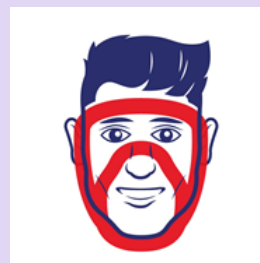
Figure 5: Example showing the face seal region that must be clean shaven for a full face mask
