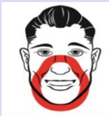
Figure 5 Example showing the face seal region that must be clean shaven for a half mask or Filtering Face Piece (FFP)
