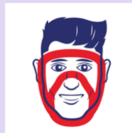
Figure 6: Example showing the face seal region that must be clean shaven for a full face mask
