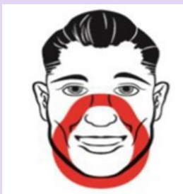
Figure 5: Example showing the face seal region that must be clean shaven for a half mask
